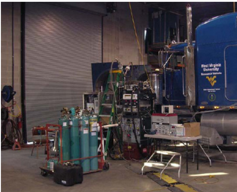
Figure 1: Peterbilt tractor with crankcase blow-by sampling system in place.
